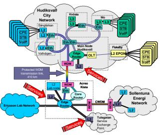
Figure 2: Schematic illustration of the testbed
